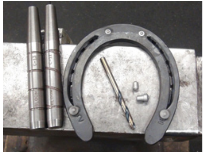
FootPro Solid Carbide Studs, Step Point Bit and Bloom Stud Set tools
