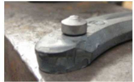
C11 applied – note the small gap between head and shoe surface.
