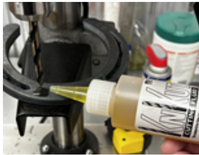
Cutting Fluid applied before drilling
