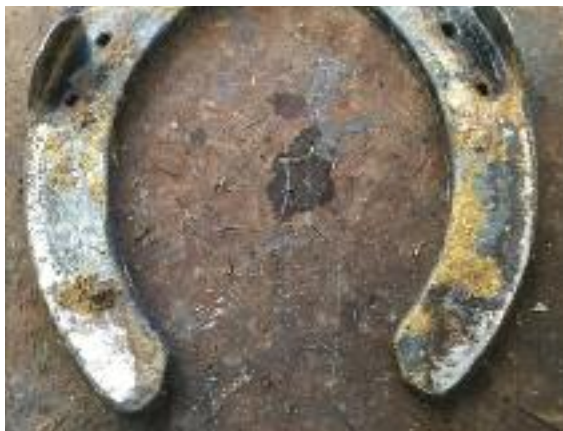
Left front shoe. Notice the wear is at and perhaps over the outer edge of the shoe from the clips back. Did the fit need to be this tight for the environment and use of the horse?
