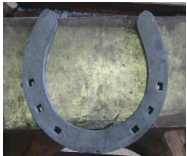
After drifting and pritcheling, make your flattening run and any last adjustments to shape.
