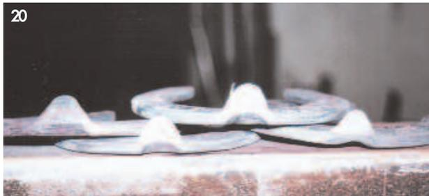
**16, 17, 18, 19.** You can see that you can get similar results no matter which tool you choose. The key to consistency is practice and hammer control. The method I use for the hammers, working from the end of the anvil, gives me a nicely balanced position where I can get good control of my hammer and the tongs. **20.** The goal is consistently strong clips no matter what method you use.
