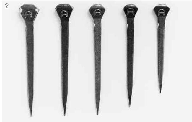
the proportionate change in the head sizes from 5 Slim to 5 Light to 5 Race. This difference in head sizes gives you some logical choices. As an example, the 5 Slim head fits well in the 5/16" thick Kerckhaert SX-8. The 5 Light will give you a better fit in the thinner SX-7. For a flush fit in the SX-7 you could choose the 5 Race. In general, the 5 Light and 5 Race will suit lighter shoes or
