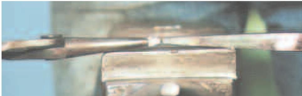
pritchel is driven in the material, the taper forces the hole to expand. The farther you go in the bigger the hole becomes. The tip of the pritchel should be backed up to produce a tip the exact size of the desired nail, leaving a slight recess behind it. By setting your pritchel in this manner, the tip will shear out the slug and the pritchel will end up in the recessed area. The pritchel will not enlarge the hole and will now also be loose in the hole.
