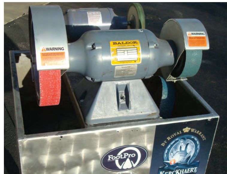
Above: Baldor Grinder with expander wheels.
