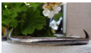
(1) Ground surface shoe wear
